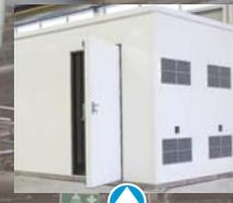
Unique composite GRP construction techniques allow INTERTEC to make lightweight shelters meeting stringent fire protection and safety requirements for offshore (or onshore) facilities - including EN 13 501-2 REI 120, UL1709 H90/H120 BS476, DIN 4102 F120. Fire resistant ceramic inner cores (below) can maintain internal temperatures below 60°C for up to 2 hours - even in hydrocarbon fires.
