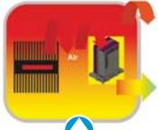
Heating (or cooling) an enclosure is a series of heat transfer processes. In this convection-heated example, thermal energy flows from heater, through the space to be heated, on to the external ambient environment through the enclosure fabric and any thermal short cuts. Optimizing enclosure materials has a highly beneficial effect.
